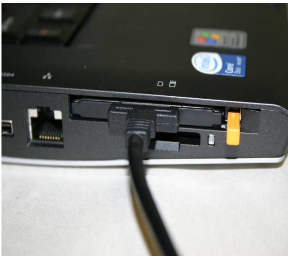
Figure 3-4, Insert PCMCIA Card into Computer
