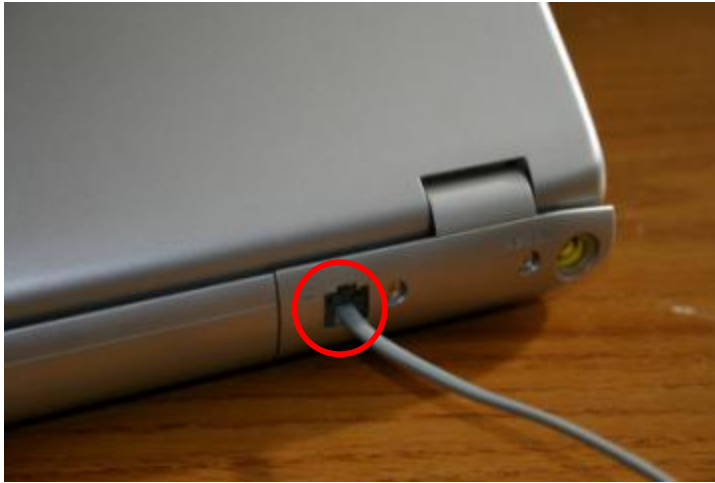
Figure 3-6, Insert Analog Line into Computer
