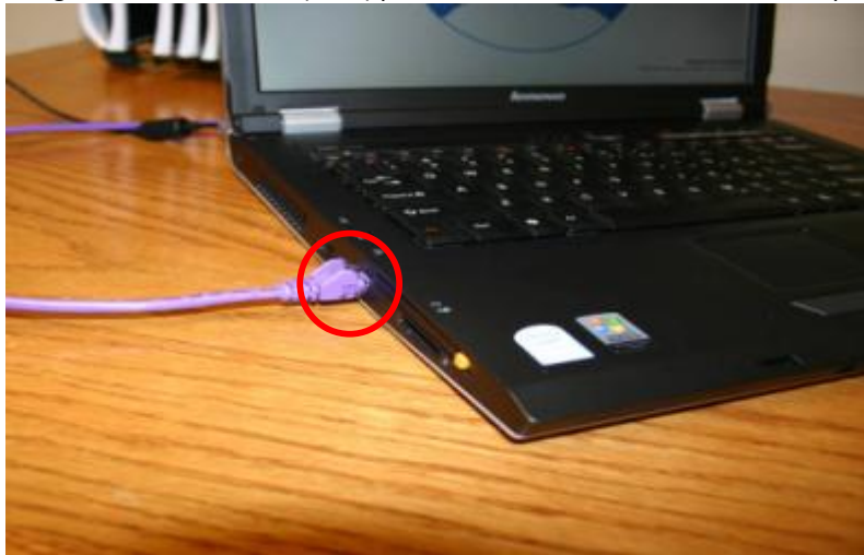
Figure 3-5, Connecting the Ethernet Cable to the Computer
